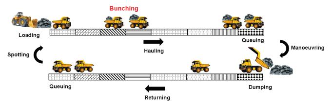
Figure 1. Schematic of hauling operation in surface mines
