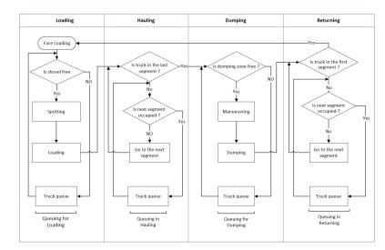
Figure 2. Truck bunching algorithm
